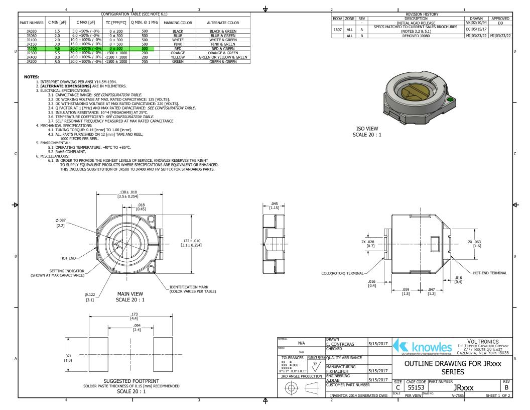
HANDLING/STORAGE PRECAUTIONS: DO NOT USE FLOW SOLDERING.
